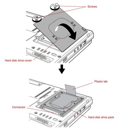
Figure 3-19 Removing the hard disk drive cover
